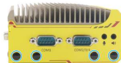
COM port panel antenna openings
