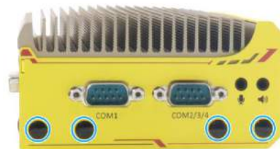
COM port panel antenna openings
