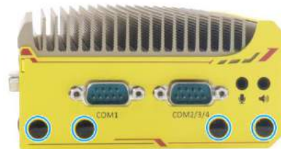
COM port panel antenna openings
