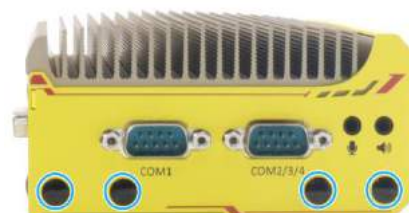
COM port panel antenna openings
