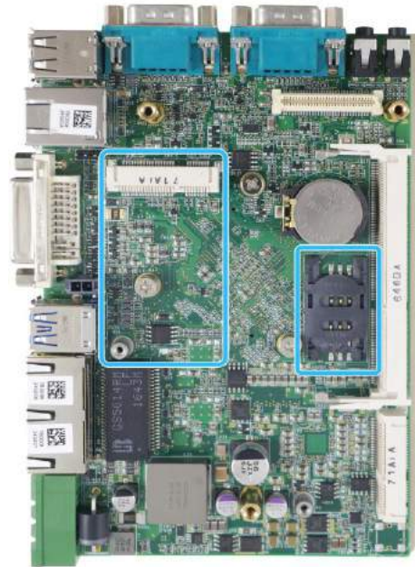
mini-PCIe/ SIM slot on the mainboard
